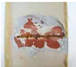
Chartek® shows low corrosion creep (<3mm)
