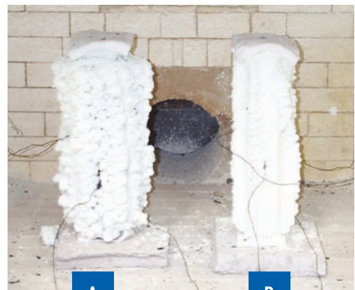
Steel columns after fire test burn, with intumesced 'char'
