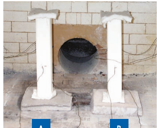
Steel columns applied with FIRETEX® FX range, before fire test burn
