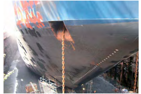
Intershield® 163 Inerta 160 – typical condition after exposure to ice, minimal damage, smooth hull
