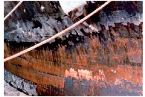
A typical standard epoxy damaged by ice - severe corrosion and very rough hull
