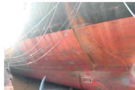
Performance on a 72,867 DWT Bulk Carrier after 60 months in-service 53% activity > 3 knots, trading globally
