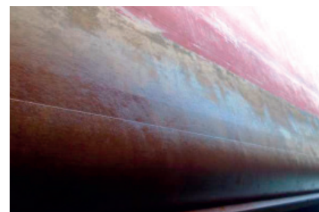
Performance on a 146,859 DWT Crude Oil Tanker after 57 months in-service 39% activity > 3 knots, trading globally
