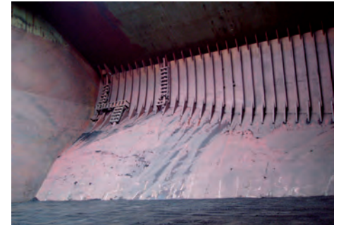
After 3 years carrying mainly coal (minimal cargo stuck to bulkheads)
